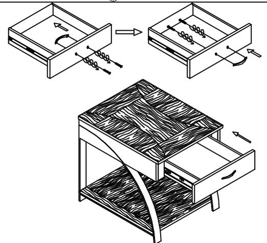
**DO NOT TIGHTEN BOLTS UNTIL COMPLETELY ASSEMBLED.**
