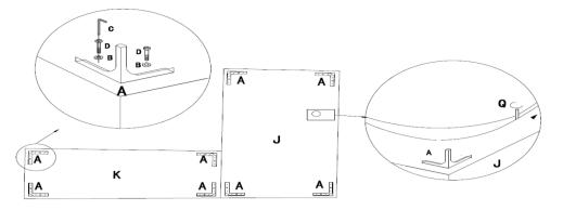
Step 2 Align and insert the back rest to the positon shown in drawing, push to the end to secure it.
