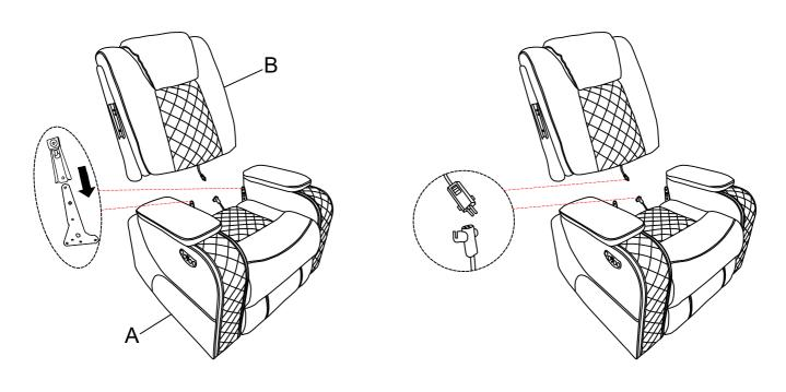
STEP 2 Insert ear to the backrest then push to the end and make sure it is fixed in position securely.
