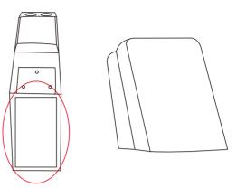
Please take out the Back(Console) from the bottom of the console. Align the holes of the Back and console, then tighten the screws in a clockwise direction.
