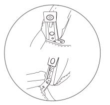
Please align the connectors of the backrest and seat according to the diagram, then press down to ensure a perfect fit.
