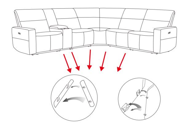
Align the connectors and connect all the items together, according to the diagram, then press down to ensure a perfect fit. Please be careful to avoid the damage to the sofa. Please check and connect the power port of seat motor and headrest motor, make sure secure the protector.
