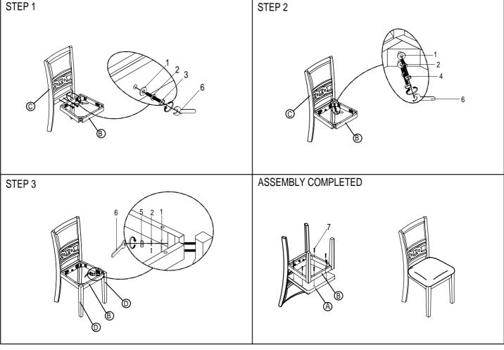
DO NOT TIGHTEN BOLTS UNTIL COMPLETELY ASSEMBLED
