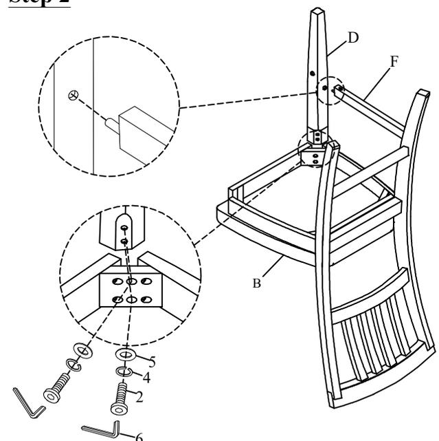
**DO NOT TIGHTEN BOLTS UNTIL COMPLETELY ASSEMBLED.**
