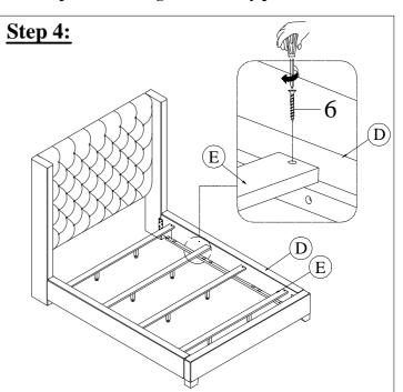
**Step 4:** Attach Slat (E) to Bed Side Rail (D) by using Screw (6) and Screw Driver (not include).
