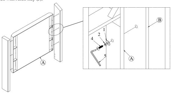
**Step 2:** Attach Rectangle Plate (8) to the Bed Side Rail (D) and H/B Side Panel (B) by using Allen Bolt (3), Spring Washer (2) and Flat Washer (1). Unfasten bolts on Footboard (C), then attach Bed Side Rail (D) to Footboard (C), tighten all bolts with Allen Key (5).
