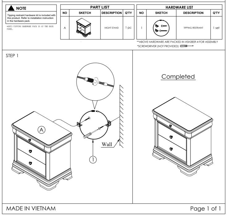
DO NOT TIGHTEN BOLTS COMPLETELY ASSEMBLED.
