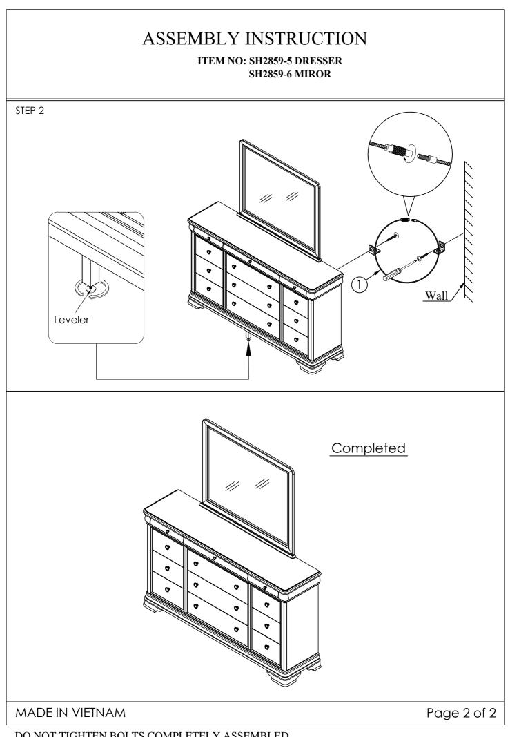
DO NOT TIGHTEN BOLTS COMPLETELY ASSEMBLED.
