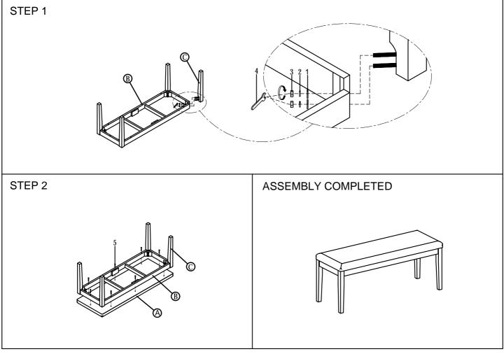
DO NOT TIGHTEN BOLTS UNTIL COMPLETELY ASSEMBLED
