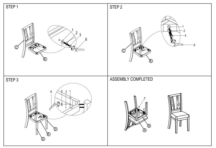
DO NOT TIGHTEN BOLTS UNTIL COMPLETELY ASSEMBLED
