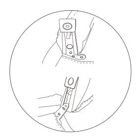
Please align the connectors of the backrest and seat according to the diagram, then press down to ensure a perfect fit.
