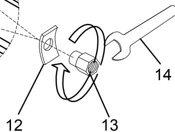
Do not tighten bolts until completely assembled.
