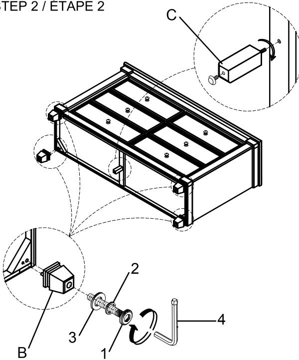
Do not tighten bolts until completely assembled
